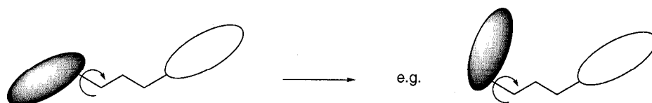
Figure 7. Influence of rotation of the mesogenic group around a meta -bond to the spacer on the ordering.
